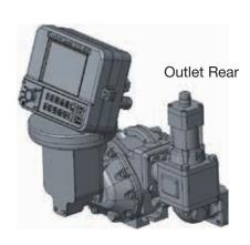
When ordered with pneumatic solenoids mounted (A26261), the valve will come pre-plumbed to the solenoids, and the solenoids pre-wired to the LCR. Air pressure, regulated to between 50 and 125psi (3.5 and 8.6 bar) must be supplied to the valve through the elbow beneath the solenoids, as shown at right. It is strongly recommended that an air dryer is incorporated in the upstream system.
