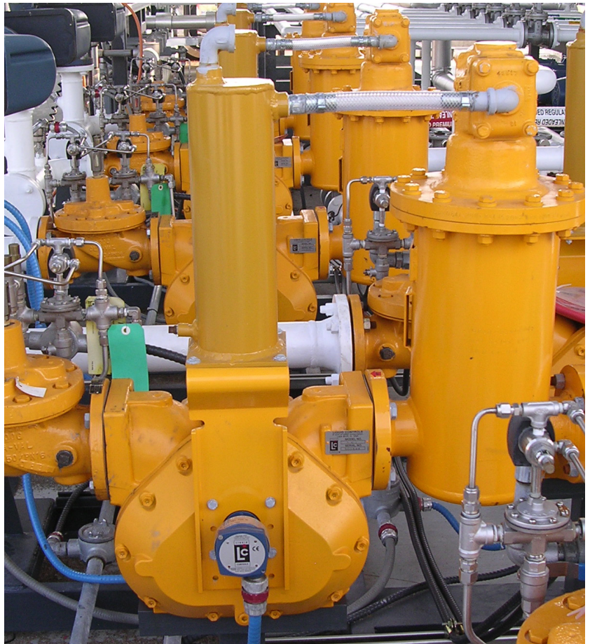
M-30 ® with LCR.iQ ® electronic register
